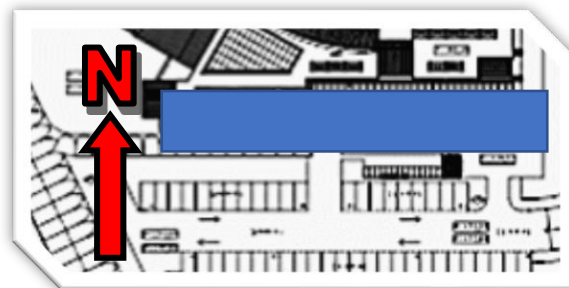
Figure 3.1: Long Directional Axis of Building (in Blue) Should Face North and South As Much As Possible
