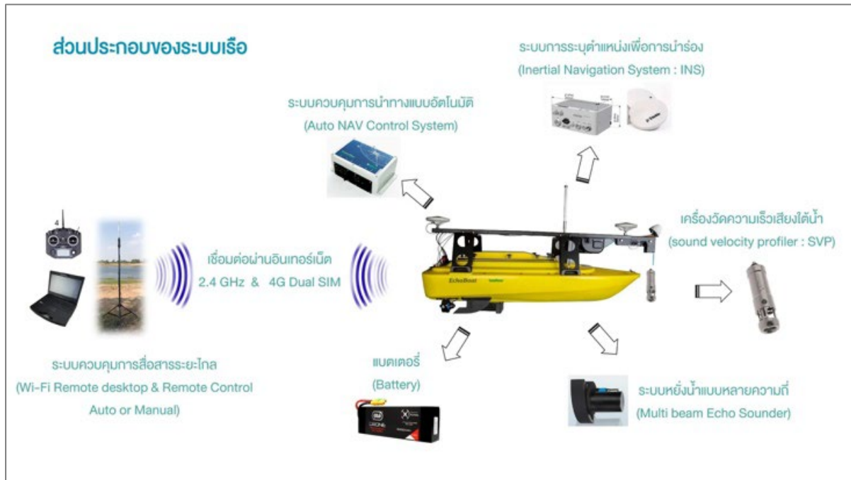
Figure 8: Components of the Automated Survey Vessel
