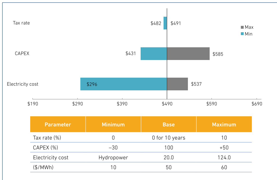
Figure 9.12. Sensitivity Analyses of the Levelised Costs of Green Urea Production in Lao PDR (US$)
