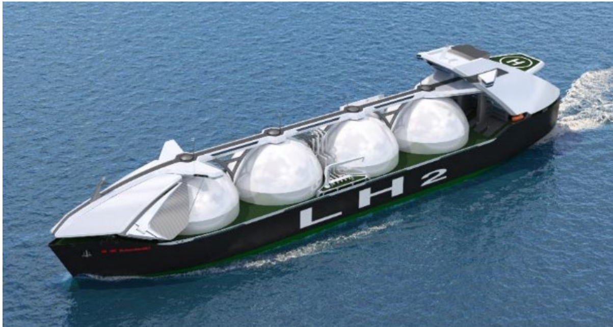
Figure 3.10. Large (16,000 cubic metres) Liquefied Hydrogen Carrier Ship (Cargo-carrying Capacity: 40,000 cubic metres × 4 tanks)
