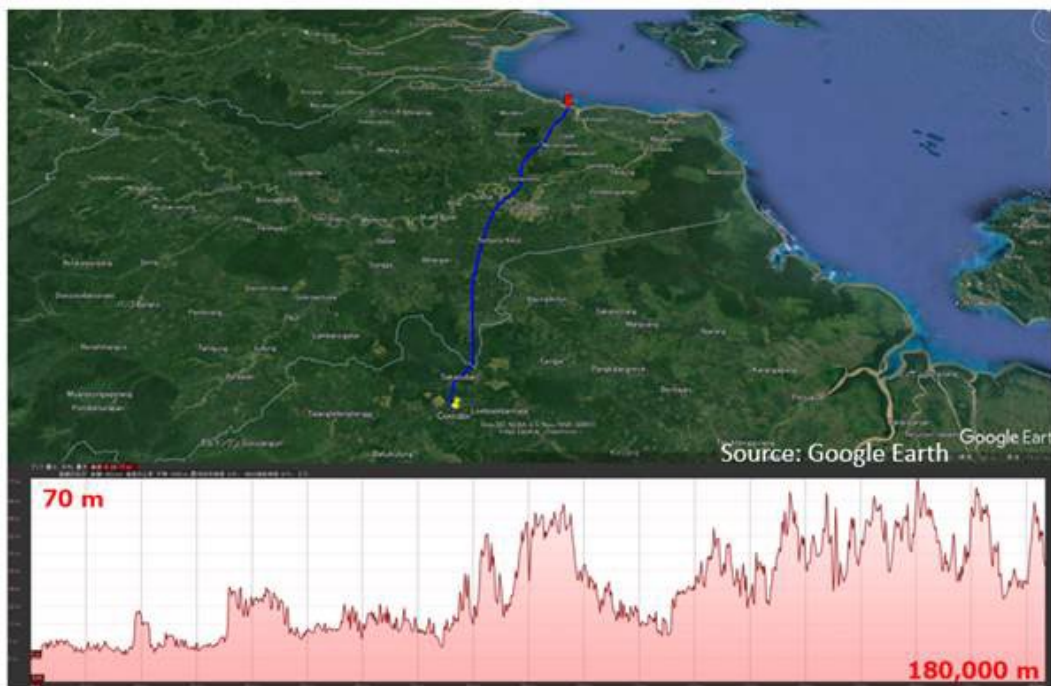
Figure 4.12. CO 2 Pipeline Route (Receiving Terminal to Corridor)
